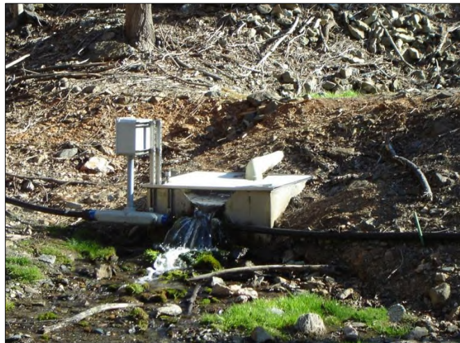
Seepage weir and collection box
